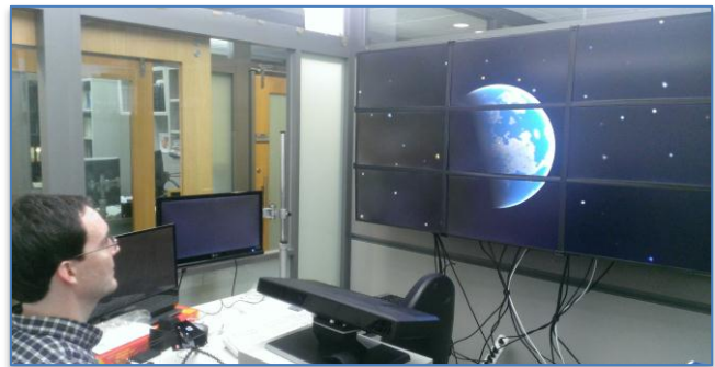
Figure 2: The tracker follows user gaze position which governs rendering to this extremely high-resolution 3x3 monitor array.
